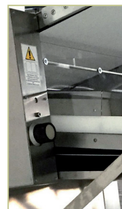
Detail of control knob for thickness adjustment
