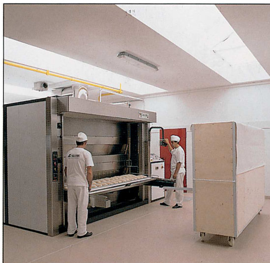
Infornamento da carrello carenato Setter loading from a faired carriage.
