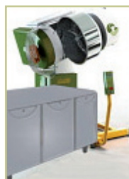
TSPI - Tipping onto worktable
